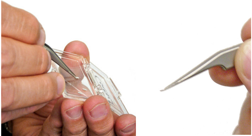
Figure 47 Holding the tweezers as shown, remove a probe from the protective case
