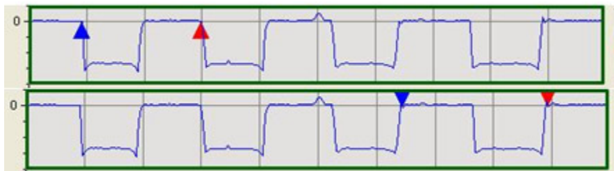
Figure 130 Cross-section in Y direction showing non-linearity
