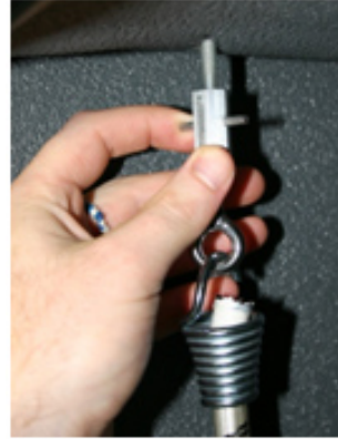
Figure 35 Adjusting bungee mounts to level the instrument platform
