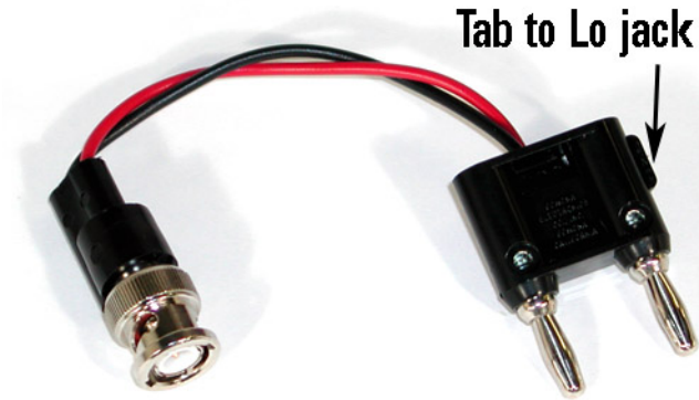
Figure 183 Tab side of Cable 3 must be inserted into the Lo jack
