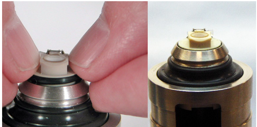
Figure 41 Apply even, vertical pressure at the edges to insert the nose assembly (as shown on left). O-ring should be fully inside socket (as shown on right).
