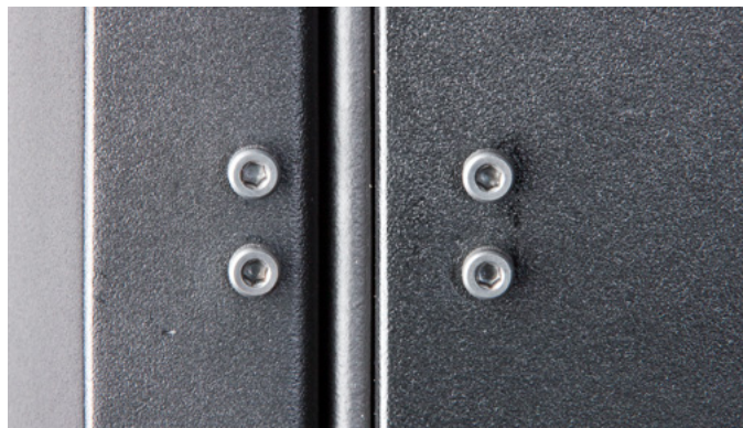
Figure 36 Fill screws on door and chamber body
