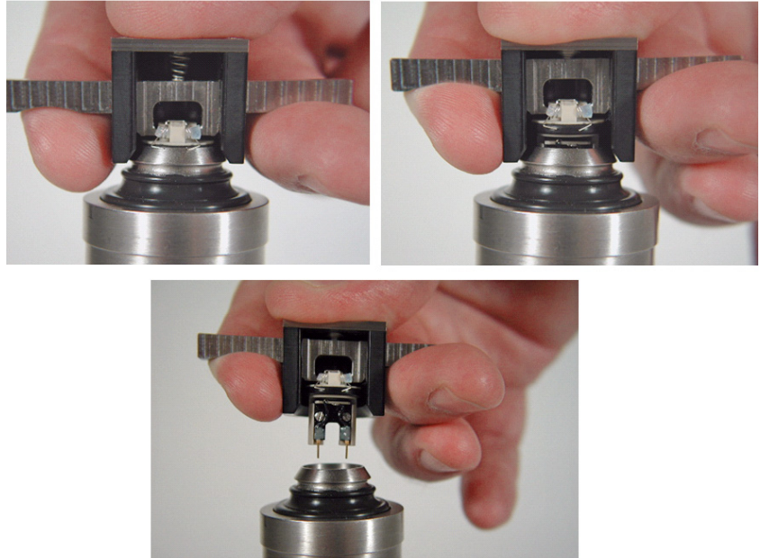
Figure 43 Using the nose assembly removal tool
