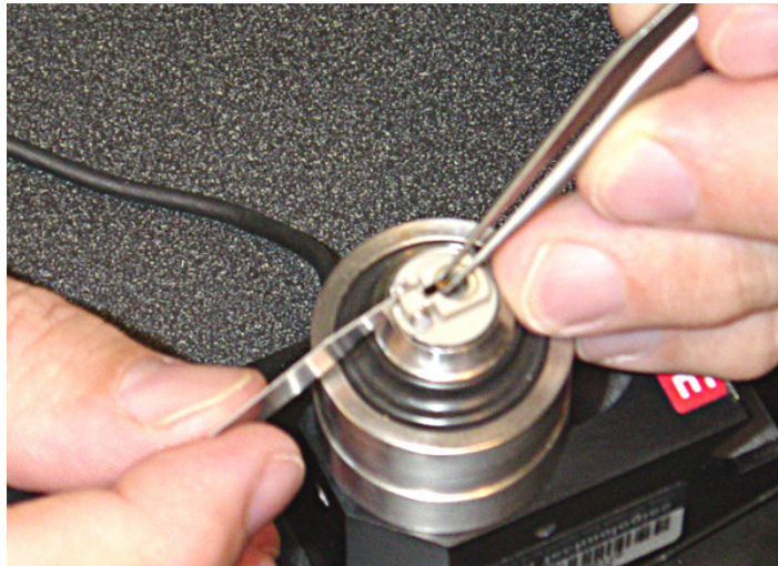
Figure 48 Hold back the retaining spring while placing the probe
