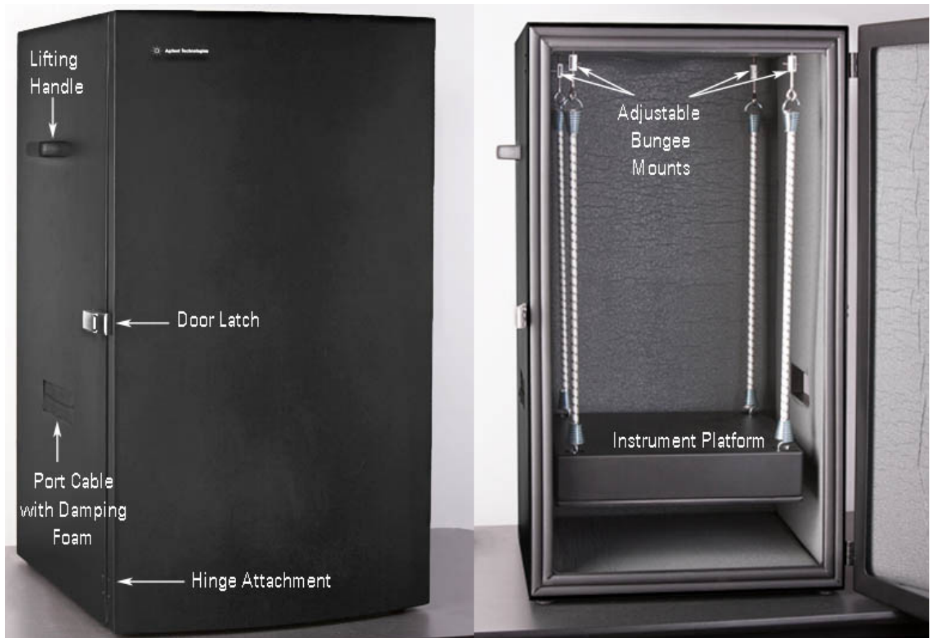
Figure 33 Vibration isolation chamber with labeled components
