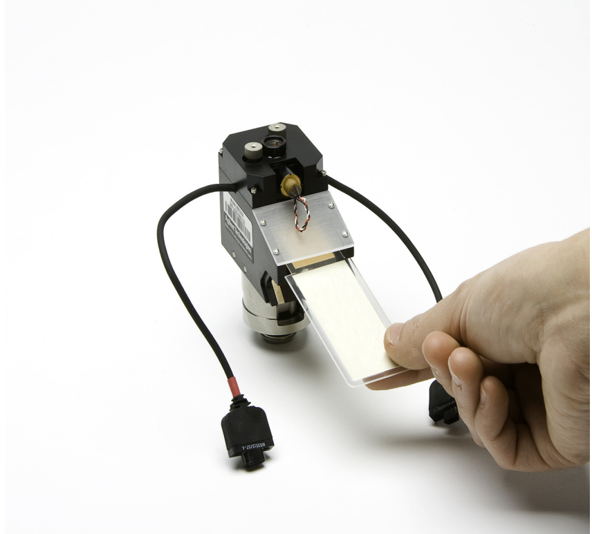
Figure 56 Coarse laser alignment for IR scanners using sensor card
